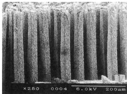
**Fig. 12.** PZT rod array (cross section:  $25 \mu\text{m}$ ).
