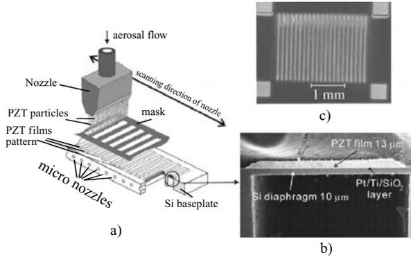
**Fig. 6.** (a) Schematic of aerosol deposition method: fabrication of micropump array, (b) Cross-sectional SEM image of 13- $\mu\text{m}$ -thick Si diaphragm, and (c) Line patterning of PZT (optical image).
