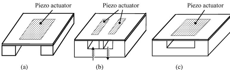
**Fig. 4.** Piezoelectric membrane actuator fabricated using micromachining technology.
