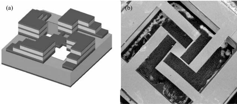
**Fig. 1.** Schematic draw of optical scanning device with double layered PZT layer (a) and the fabricated device (b), Mirror plate:  $300 \times 300 \mu\text{m}^2$ , DPZT beam:  $800 \times 230 \mu\text{m}^2$ .
