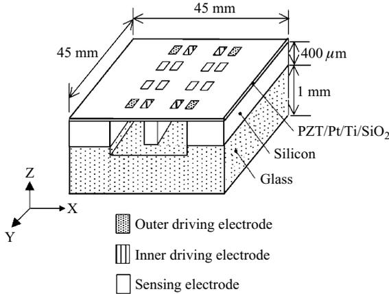
**Fig. 9.** PZT film angular rate sensor using a membrane type actuator
