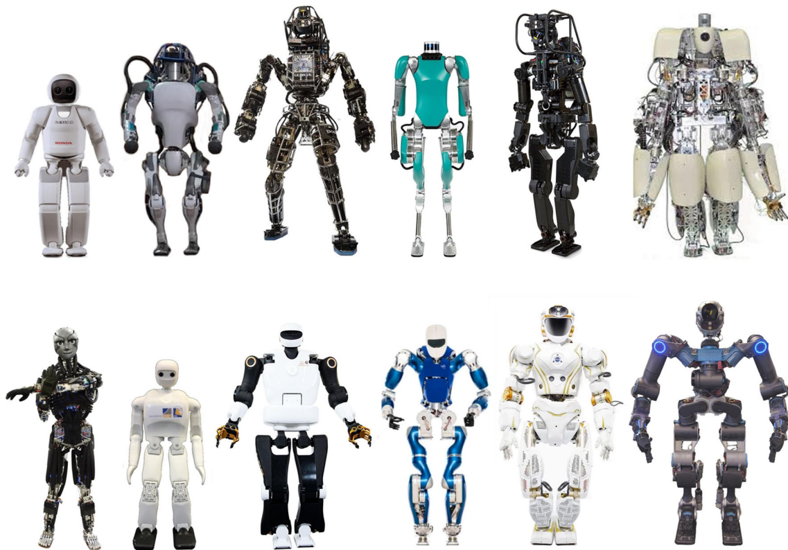
Fig. 1 Most recently developed bipedal humanoid robots with a full humanoid body plan, from left to right, top to bottom: Asimo, Atlas, Atlas-Unplugged, Digit, HRP-5P, Hydra, Kengoro, Nimbro-OP2X, TALOS, Toro, Valkyrie, WALK-MAN
