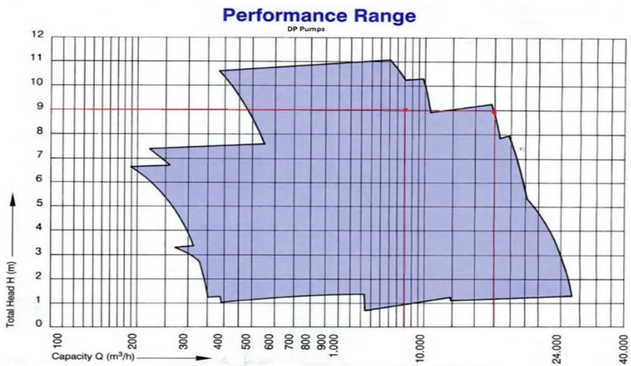
Fig. 16 DP Pump performance diagram (head/capacity) [37]
