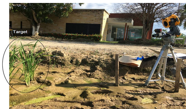
Fig. 13 Plant image acquisition, in field conditions, with plenoptic, multispectral and thermal cameras configuration
