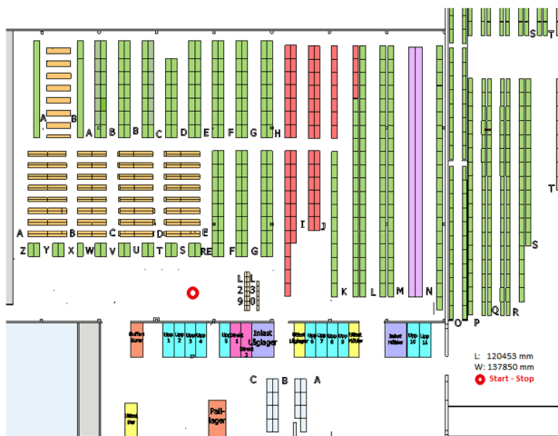
Fig. 4 Top-view of the Aba Skol AB warehouse. The picking zones are color-coded. The red circle denotes the most commonly used depot location
