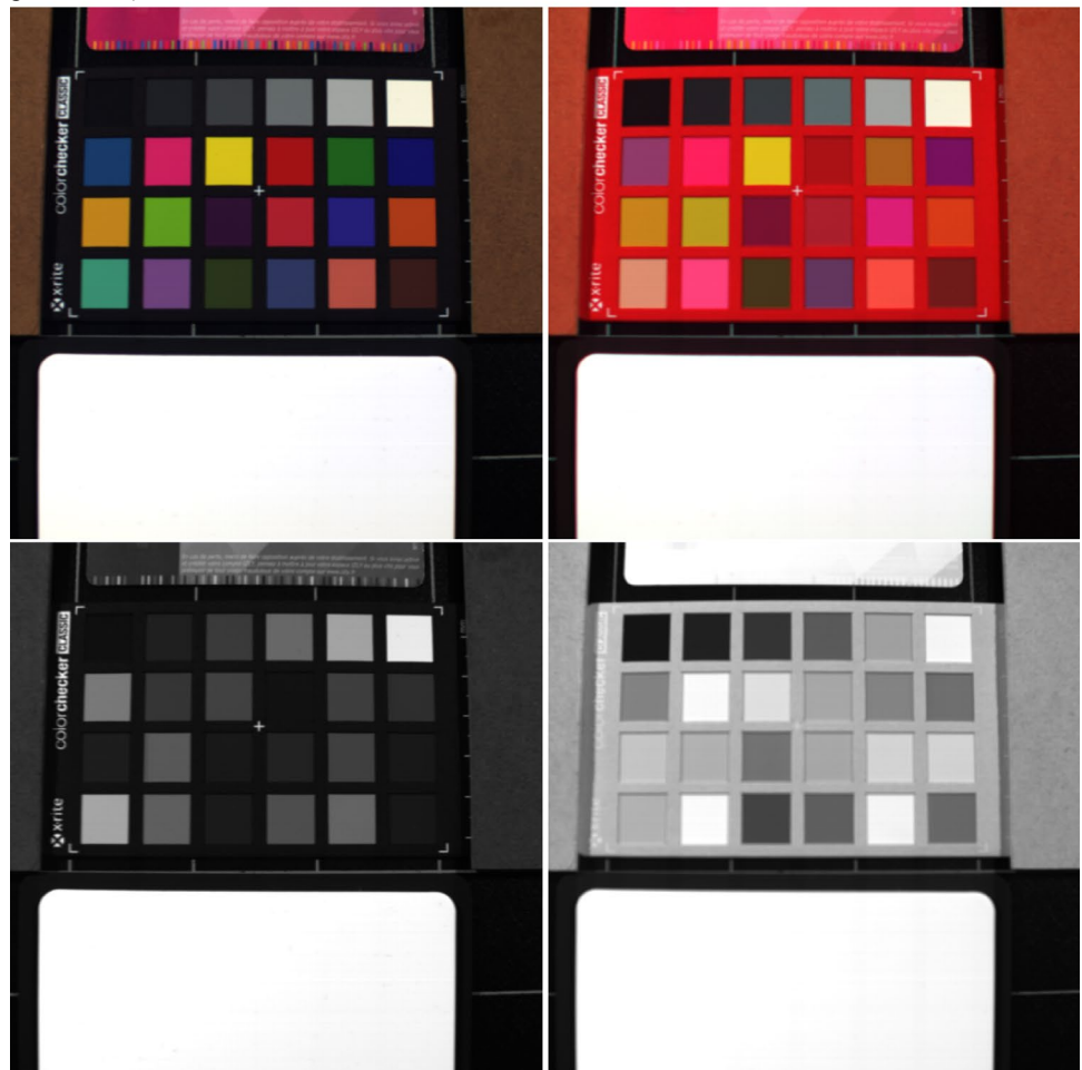
(b) Wavelength reconstruction - \lambda_R=650 nm, \lambda_G=550 nm, \lambda_B=450 nm (upper left) - \lambda_R=900 nm, \lambda_G=550 nm, \lambda_B=450 nm (upper right) - \lambda_R=500 nm, \lambda_G=500 nm, \lambda_B=500 nm (bottom left) - \lambda_R=850 nm, \lambda_G=850 nm, \lambda_B=850 nm (bottom right)
