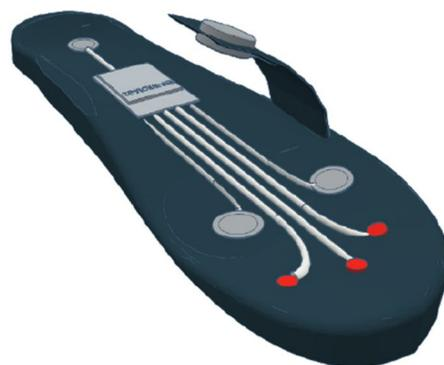
(a) 3D model of *SmartInsole*
