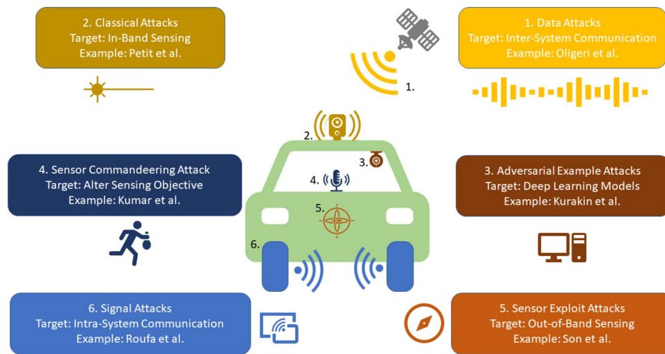
Fig. 1 Examples of different attacks on an autonomous vehicles as classified by our lexicon. 1 Refers to the GPS data spoofing attack as described by Oligeri et al. 2 Is the classical spoofing/jamming attack on lidar as conducted by Petit et al. against lidar. 3 Represents algorithmic attacks generated by Kurakin et al. for deep learning image
