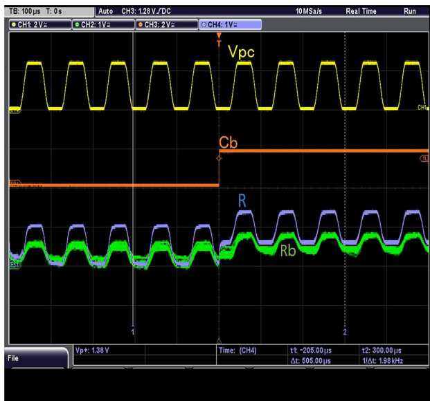
Fig. 9 Transient waveform of 4-bit QUALPUF at 10 kHz
