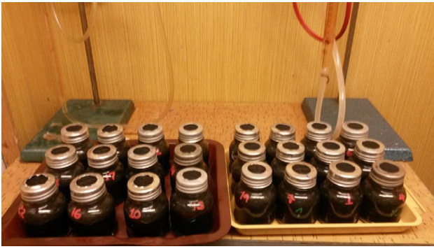
Fig. 1 Setup of the biochemical methane potential assay
