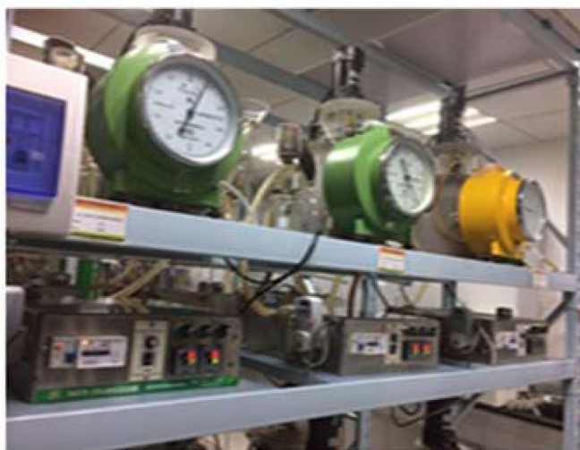
Fig. 2 Experimental setup for CSTR digester. 1: influent point, 2: mixer (stirrer), 3: temperature sensor, 4: rpm controller (stirrer motor), 5: biogas volume measuring meter, 6: effluent outlet, 7: hot water jacket
