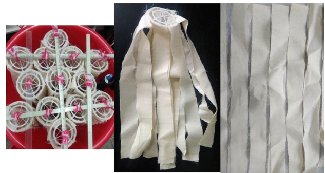
Fig. 2 Images of WCC strips used to make the biofilm carrier showing WCC strips (right), the biofilm carrier unit (middle) and those hanging in the reactor (left)
