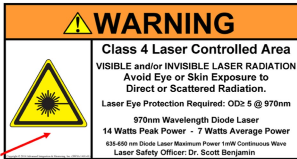
Fig. 3 Warning signs when diode laser is in use should be posted at the entrance to the dental operator
