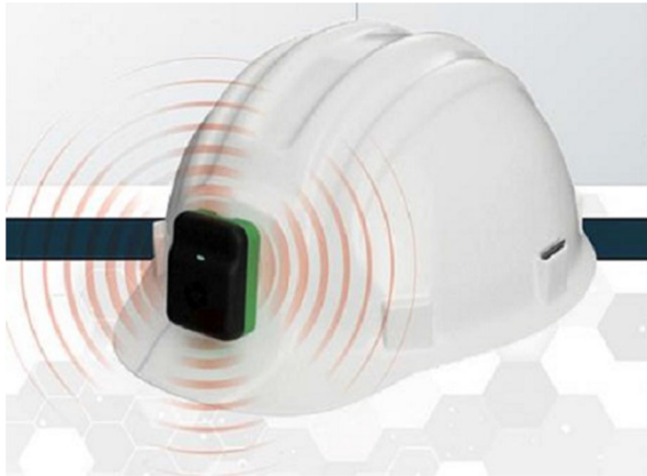
Fig. 18 Use of TraceTag on a hard hat [37]
