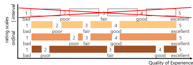
Fig. 1 The ACR scale is just an ordinal scale, not an interval scale. Differences between rating categories might not be equidistant. Moreover, differences between the categories might be different for each participant
