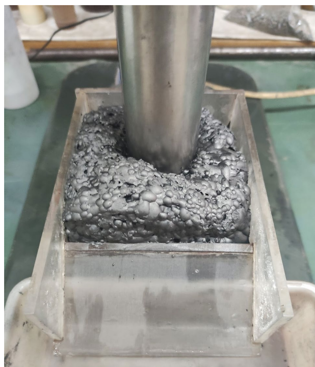
Fig. 3 Graphite froth flotation
