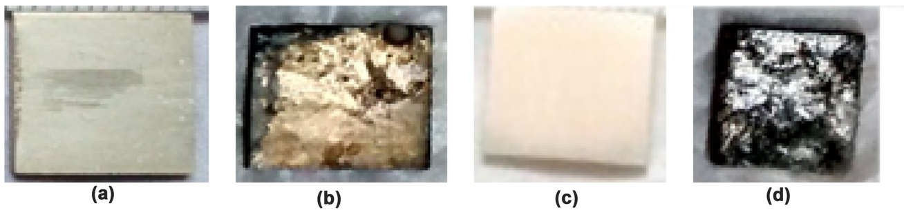
Fig. 4 Photographs of AZ-ACP before immersion (a), after immersion (b), AZ-U sample before immersion (c), after immersion (d)
