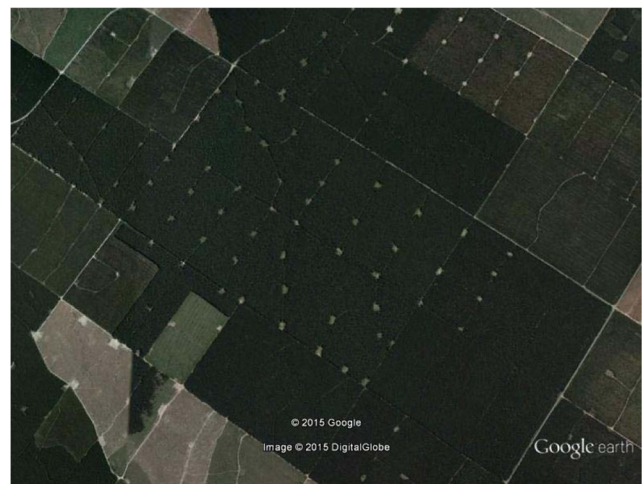
Fig. 1 An example of road and landing spacing for plantation forests on New Zealand's North Island [used with permission via Google's guidelines]
