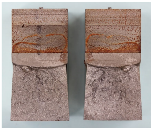
Fig. 9 Fracture faces from the carbon steel SENB specimen giving a fracture result after achieving CTOD of 0.9 mm
