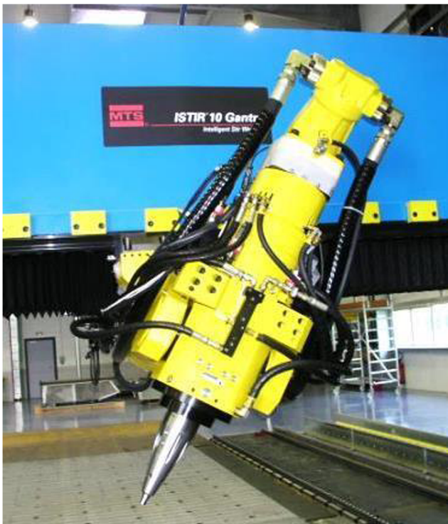
Fig. 34 FSW head of the huge IS gantry machine [41]
