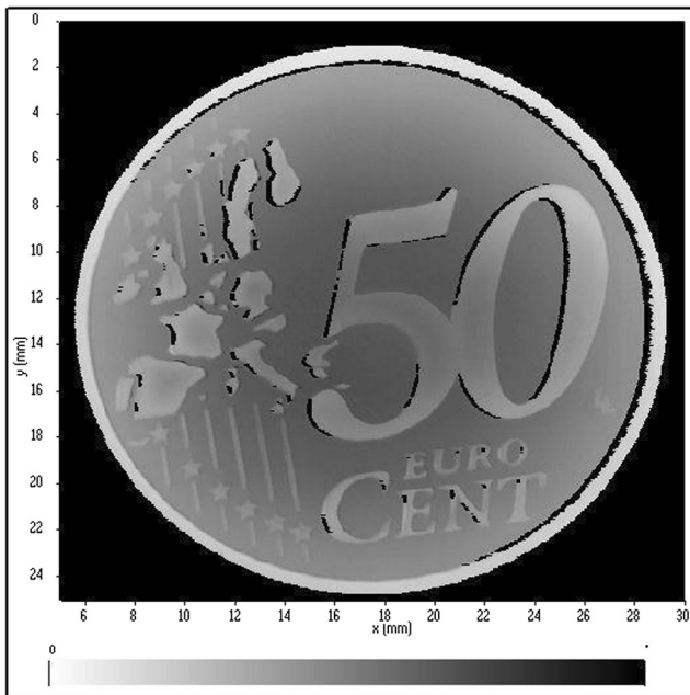
Fig. 12 HF UT C-SCAN on a coin
