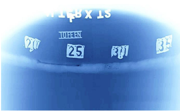
Fig. 7 CR image on a weld after basic image processing
