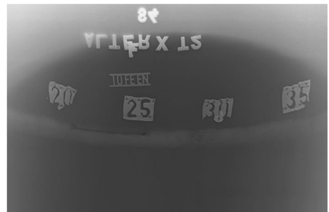
Fig. 6 Raw CR image on a weld
