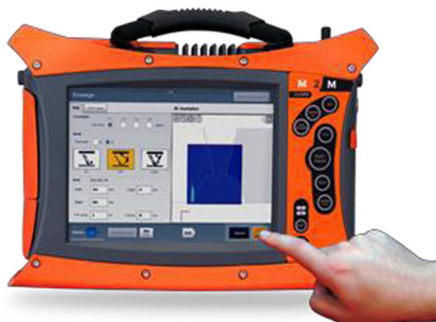
Fig. 21 Example of portable equipment able to perform TFM/FMC in real time
