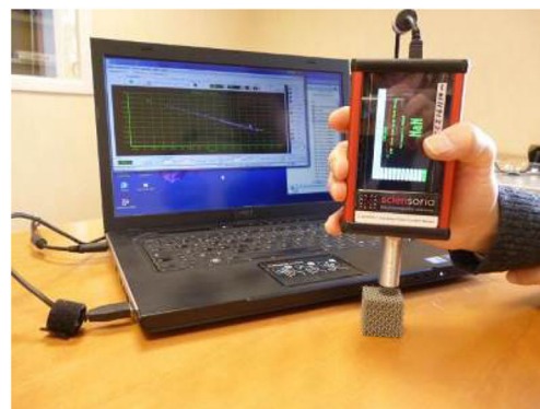
Fig. 9 Sciorsoria eddy current system used to measure the studied parts in electrical conductivity
