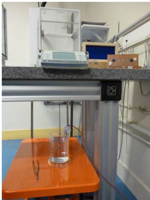
Fig. 1 LNE Archimedes' method setup used to measure the studied parts in density
