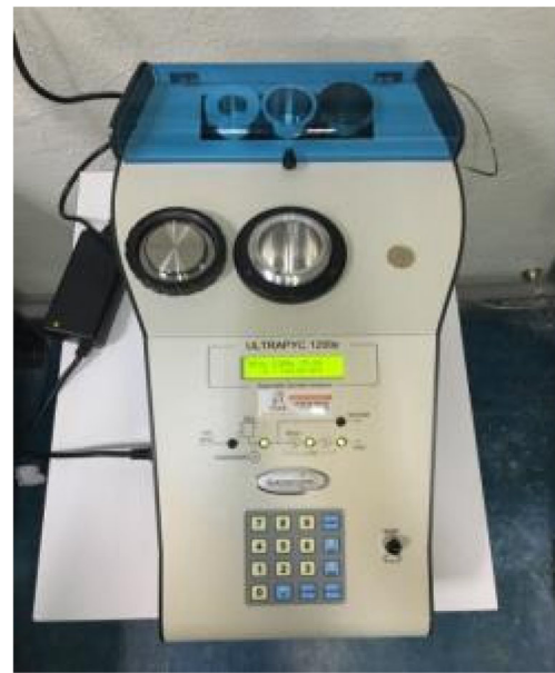
Fig. 6 LNE pycnometer used to measure the studied parts in volume
