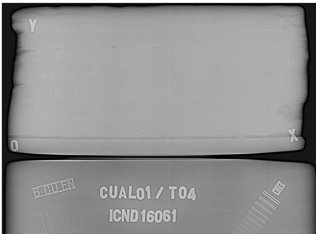
Fig. 10 Radiographic test on a Cu-Al8Ni2Fe2 multipass block
