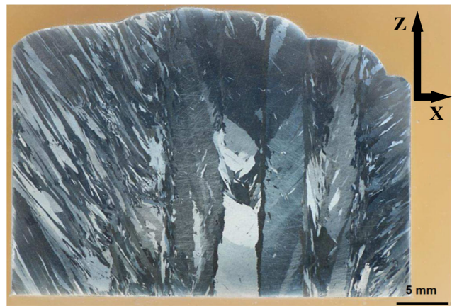
Fig. 12 Cross-section macrography on a Cu-Al8Ni2Fe2 multipass block
