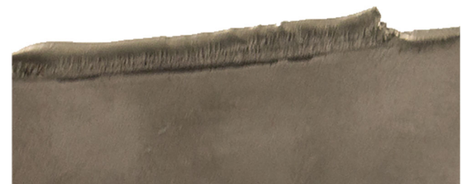
Fig. 12 Multi-layer deposition (3 layers)
