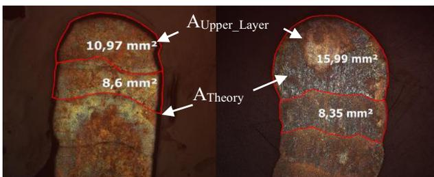
Fig. 6 Definition of the areas of the different welds (left: 3DPMD; right:CMT)
