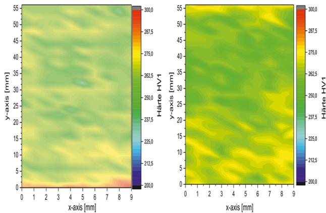
**Fig. 8** Hardness mapping (left: 3DPMD; right: CMT)
