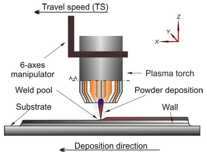
Fig. 1 Process setup 3DPMD
