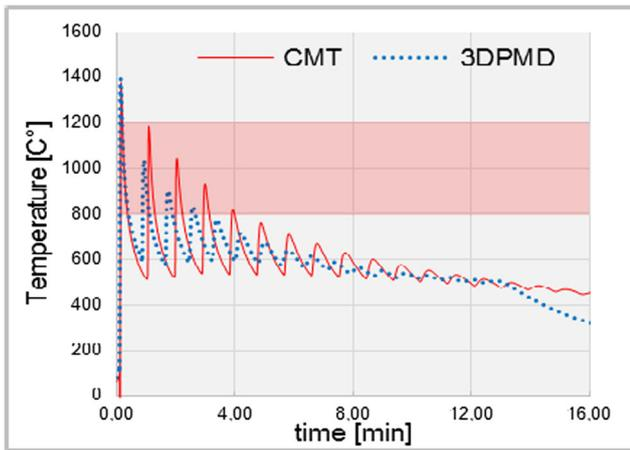
Fig. 5 Cooling chart of the processes
