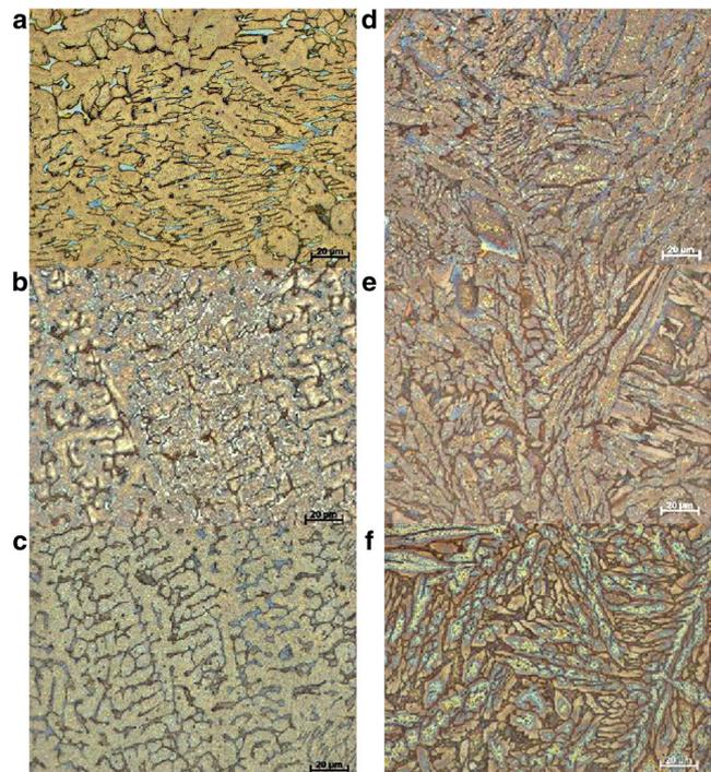
Fig. 7 Build-up of the welds. **a** 3DPMD, top of the part; **b** 3DPMD, middle of the part; **c** 3DPMD, below the part; **d** CMT, top of the part; **e** CMT, middle of the part; **f** CMT, below the part
