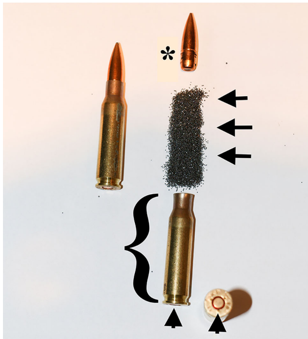
Fig. 3 Anatomy of a bullet. On the left is a 7.62 mm NATO FMJ rifle round. On the right it has been broken down into its components the projectile (*), the charge (solid arrow), the casing (bracketed) with primer (arrowheads)
