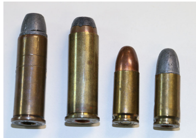
Fig. 4 Different types of bullets: From left to right, a Non-Jacketed .44 magnum, a Semi-Jacketed .44 magnum, a full metal jacket 9 mm and Non-Jacketed 9 mm
