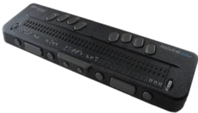
Fig. 4 Classic Focus 40 Blue device that converts text into Braille in real time
