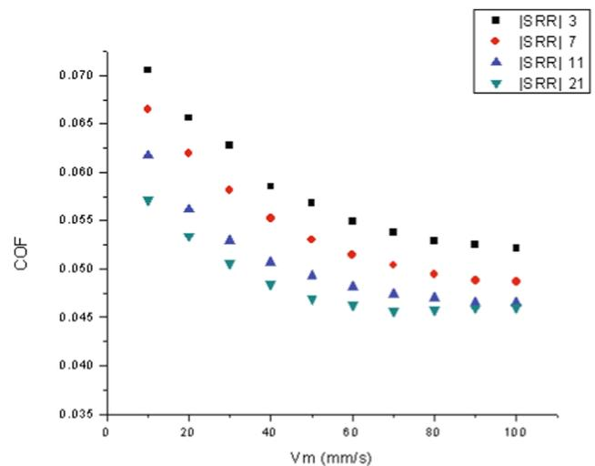
**Fig. 3** Typical Stribeck curves for the maximum contact pressure  $P_m = 19.1$  MPa
