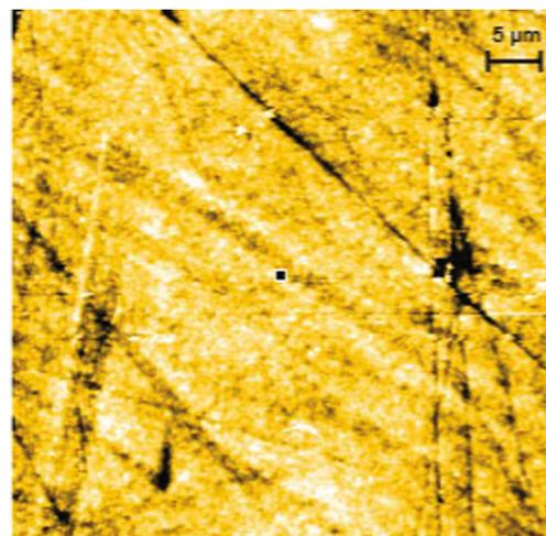
**Fig. 2** Surface topography of the polished UHMWPE surface measured by AFM
