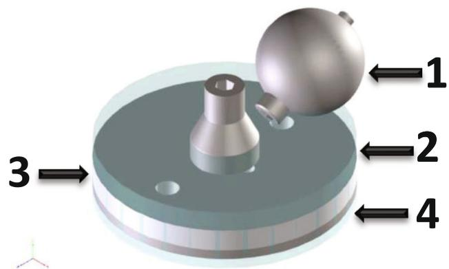
**Fig. 1** Schematic representation of ball-on-disc tribometer. (1) AISI 316L ball, (2) Lubricant, (3) UHMWPE disc, and (4) AISI 316L support
