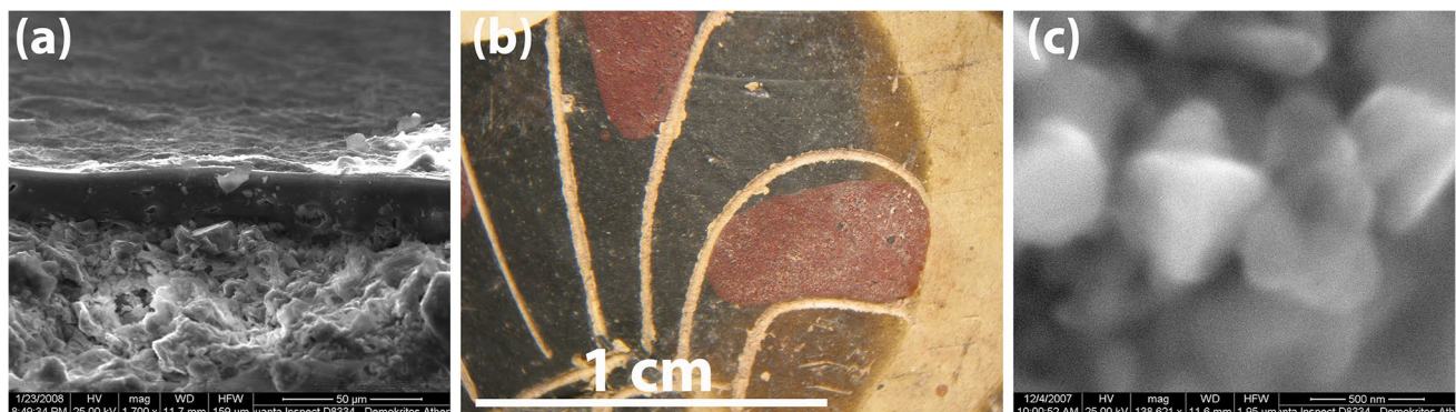
Fig. 5 a Vitrified black gloss layer on top of a ceramic body; archaic pottery sample (Greece, sixth century BCE), SEM image, magnification 1,700×. b Black gloss decoration, partially covered by deep red
