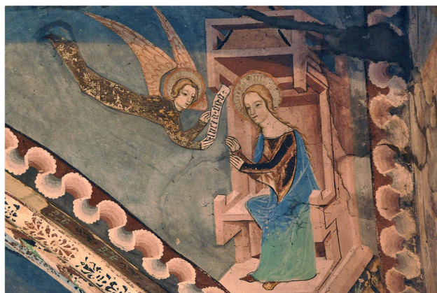
Fig. 8 Photograph illustrating the colour change of Virgin Mary's drapery from blue to green under action of chlorides on the wall painting in the church of Virgin Mary in Mălâncrav, Transylvania, Romania (photo D. Hradil). Adopted from Švarcová et al. (2012)
