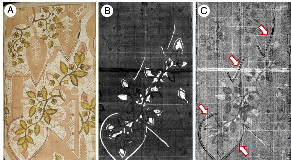
Fig. 3 (A) Design 73 from the V&A Leman album (accession number E.1861:73–1991) and images created after hyper-spectral imaging experiments, emphasising which areas of later interventions have been painted with lead white (B) and where a dark ink has been used to outline some of the details (C, marked by red arrows). Experiments made in the framework of Iperion-CH grant n. 654,028, see Manca et al. (2019) for the experimental details
