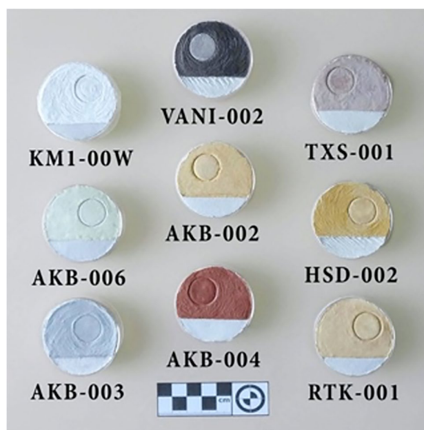
Fig. 3 Preparation of some of the samples as pigments for frescoes (see Fig. 2b and Appendix 2). VANI=VAN-002
