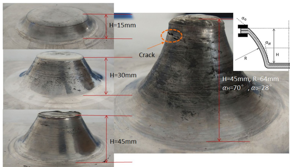
Fig. 8 The fabricated laminated parts with different shape design
