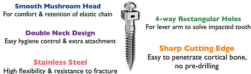
Fig. 2 Design specifications for a 2 × 12-mm stainless steel bone screw (OrthoBoneScrew®). The 12 mm length is suitable for the MBS and IZC, but a 14-mm screw is required for mandibular ramus screws (MRS) because of the thick soft tissue covering the osseous site
