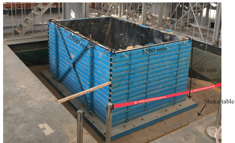
Fig. 4 Laminar shear box used for the test at IEM, CEA, Hebei, China
