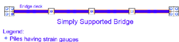
Fig. 19 Hatching marked piles have strain gauges attached at different elevations
