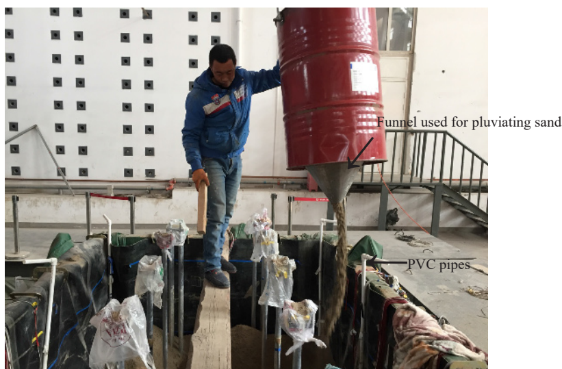
Fig. 6 Photograph of preparation of the sand layer in the test and PVC pipes being used to put the water inside
