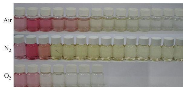
Fig. 4 The color of AF solution (1 L, 100 mg/L) after being treated by the plasma bed with a power of 90 W, water flow of 50 mL/min and gas flow of 5.0 SLM (solution in each bottle was diluted by 20 times). The corresponding processing time of each bottle from left to right was increased by 15 min starting from 0 min (original AF solution)
