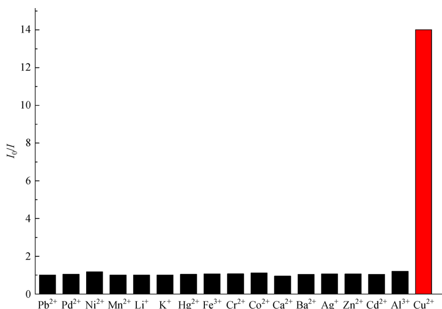
Fig. 1 Fluorescence quenching efficiency of PFPNCC ( 1.0 \times 10^{-6} mol/L) in DMF by adding metal ions. \lambda_{\text{ex}} = 370 nm, \lambda_{\text{em}} = 420 nm. C_{\text{Metal ion}} = 4 mmol/L
