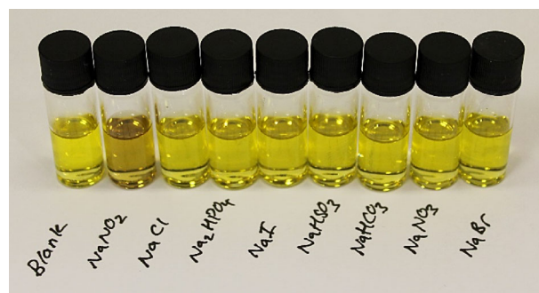
Fig. 5 Selectivity of azulene probe 9 and various anions in solution after 10 min. Each vial contains a mixture of MeCN (0.4 mL), DI water (0.1 mL), \text{HCl}_{(\text{aq})} 35% (0.3 mL), sensor 9 (0.1 mL, 5 mmol/L in MeCN) and analyte (0.1 mL, 5 mmol/L in DI water)
