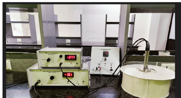
Fig. 5 Experimental setup of thin film gas sensor for measuring response toward H 2 S gas.
