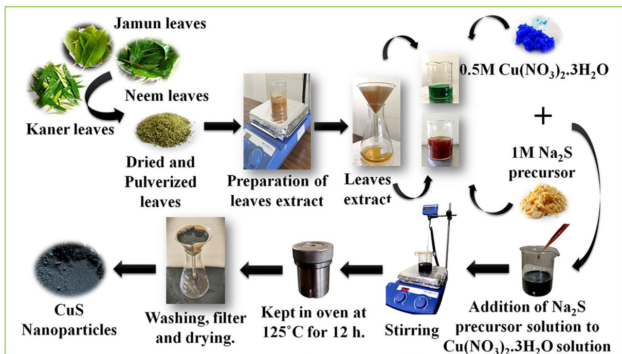
Fig. 1 Synthesis route for synthesizing CuS nanoparticles using leaf extracts of neem, jamun, and kaner.
