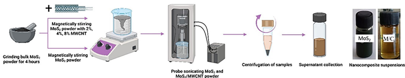
Fig. 1 Synthesis process of pristine MoS 2 and MoS 2 @MWCNT composite nanosheets.
