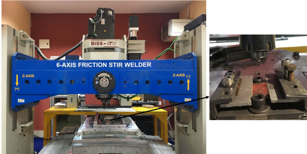
Fig. 2. Picture of FSW machine, and fabricated fixture.
