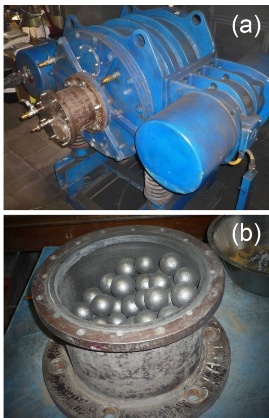
Fig. 1. Eccentric vibratory mill with attached satellite (a), and open satellite filled with milling balls (b).
