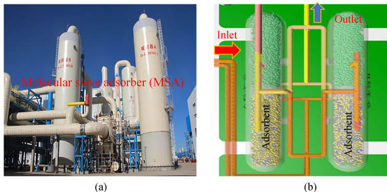
Fig. 5 MSA. (a) Two vertical radial flow MSAs; (b) simulation process of MSAs.
