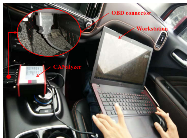
Fig. 16 Test data acquisition.
