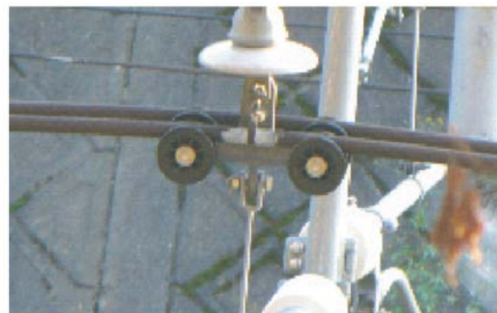
Fig. 5 Temperature-induced tension decreasing in the catenary and the solution. (a) Messenger wire's tension versus temperature; (b) messenger wire supporting pulleys
