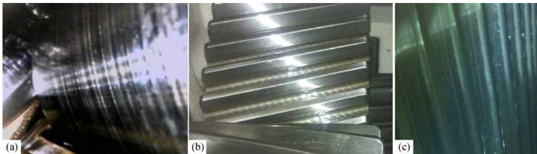
Fig. 4 Machine faults in transmission systems of wind turbines. (a) Scratches on bearing race; (b) spalls on gear teeth surface; (c) abrasion on gear teeth top
