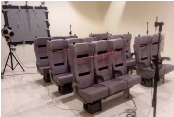
Fig. 2 Absorption coefficient test of the sound-absorbing seats
