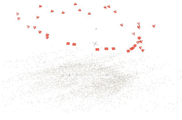
Fig. 10 Approximate poses recovered by using COLMAP on the scene centered around a reflective fork object (Sect. 4.3.2), proposed in Yen-Chen et al. (2022b)
