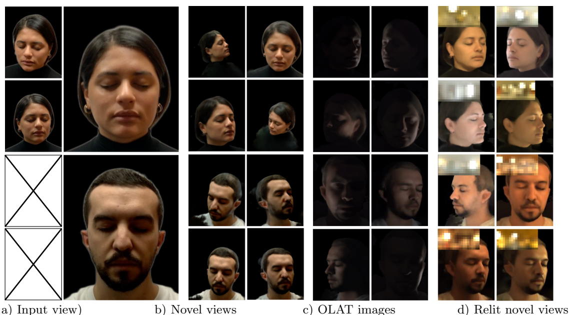
Fig. 1 We present VoRF, a learning framework that synthesizes novel views and relighting under any lighting conditions given a single image or a few posed images. VoRF has explicit control over the direction of a point light source and that allows the rendering of a basis of one-light-
