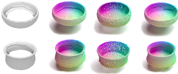
Fig. 10 Results on point clouds from real pottery objects. From left to right: the first column shows the partial input, the second column shows the results of MSN (Liu et al., 2020), the third column shows the results from VRCNet (Pan et al., 2021), and the fourth column shows the results from our method
